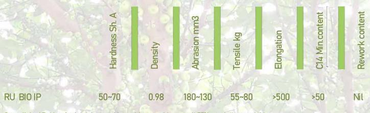
Cross linked Rubber for injection machine with vegetal base until 55%, partially recyclable
